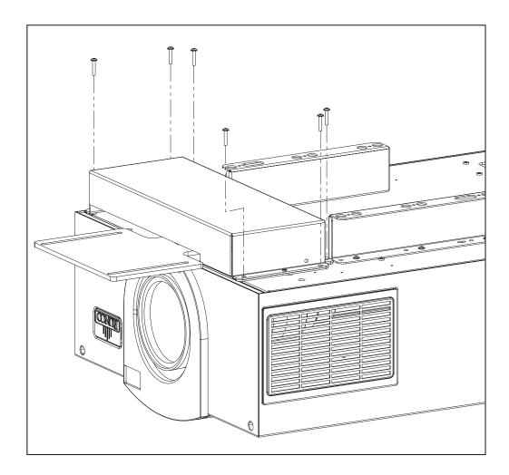
Figure 3-8. AutoScope Lens Motor Installation
